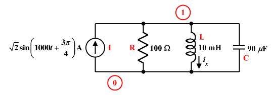
the following LTspice netlist can be used determine the magnitude and phase angle of the steady-state AC part of  $i_x$ :
